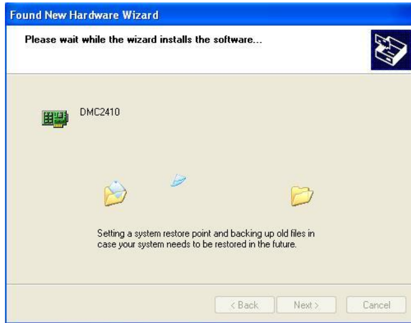
Figure 2-4 Driver is installing
