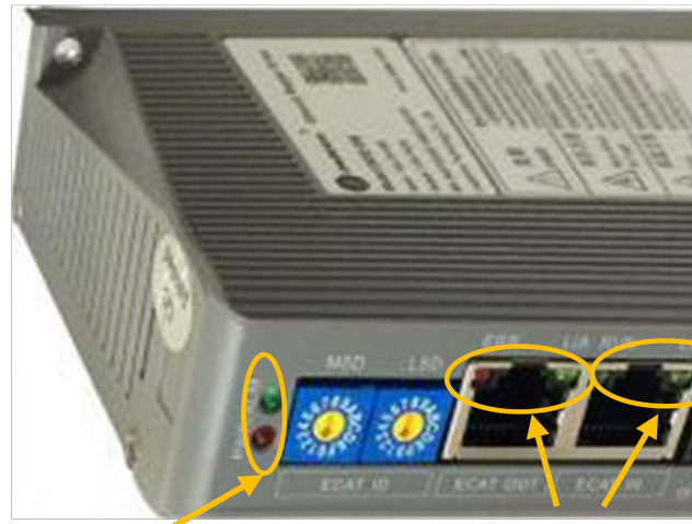
L1: Power/Alarm Indicator L2: EtherCAT Communication Indicator
