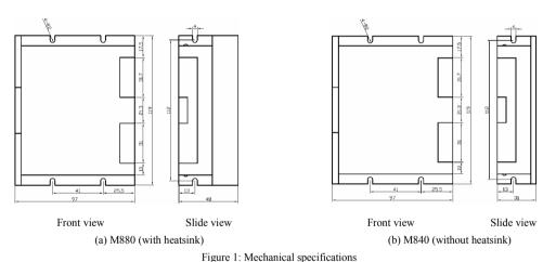
Figure 1. Mechanical specifications
