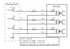
Figure 4: Connection to PNP signal (common-cathode)
