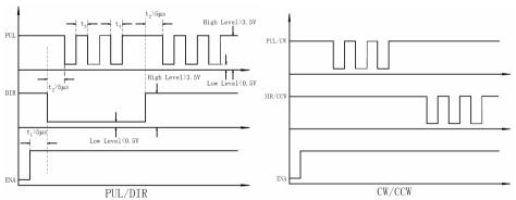
Figure 11: Sequence chart of control signals
