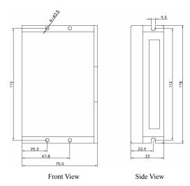
Figure 1: Mechanical dimensions
