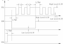
Figure 10: Sequence chart of control signals
