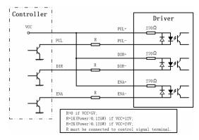
Figure 3: Connections to open-collector signal (common-anode)
