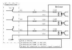
Figure 4: Connection to PNP signal (common-cathode)
